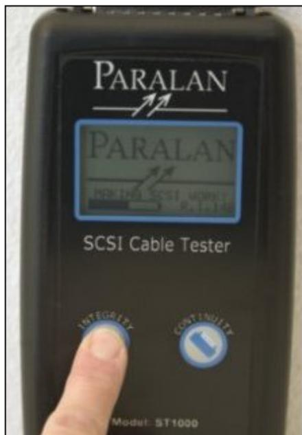
The ST1000 SCSI Cable Tester is designed with an emphasis on simplicity of use. Connect a cable, press a switch and the LCD indicates the test results within 5 seconds. In addition to Continuity and Integrity, the ST1000 also tests to determine that the critical REQ and ACK signal pairs are located in the inner layers of the cable.
