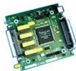
The board-level version Model MH33A is sized to fit in a standard 3.5" drive bay
