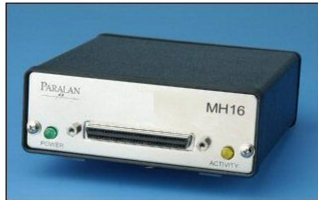
*The stand-alone Model MH16A includes a power supply for standard power line operation*
