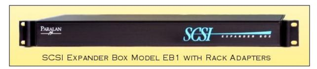
The Model EB1 includes positions for mounting and powering up to three SCSI expanders, which may all be the same or may have a different type of expander in each postion. All I/O connectors and the connector for the power cord are on one side of the box. Each expander has a "Power" and an "Activity" LED. All expanders are powered by one internal auto-ranging line voltage operated power supply. The power supply has an IEC line voltage power connector and includes an on-off switch.
